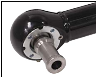
Offset Pivotball for narrowed mini-tub configuration.
